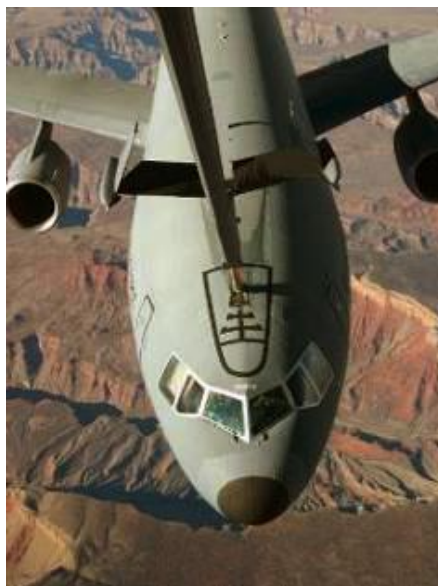
Figure E-4. Triple Bar Camouflaged Receptacle Markings
